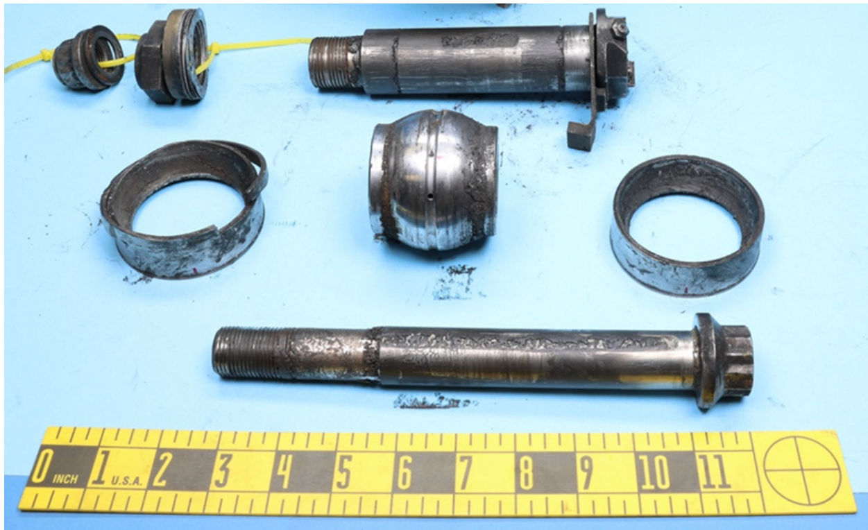
Figure 10. The spherical bearing and attachment hardware after removal from the left wing clevis.
